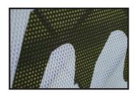
Heavy mesh material keeps wind blowing through
